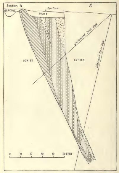
Fig. 14-A.—Mandy mine, Schist Lake, Manitoba, Canada. Vertical crosssection. For legend see Fig. 14-B, p. 113.
